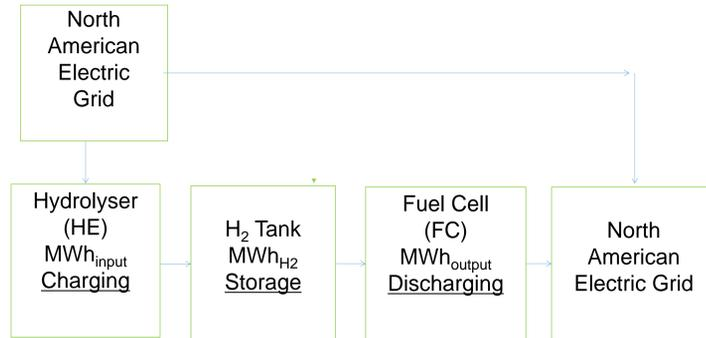
Schematic of a Hydrogen Storage Plant (HSP) on the North American Grid
