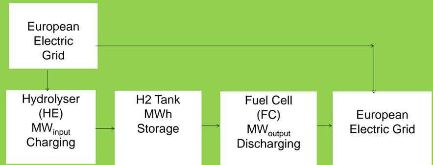
Schematic of a Hydrogen Storage Plant (HSP) on the European Grid
